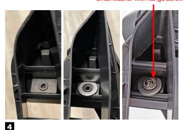
Flip everything over, then place the clipped washer, as shown in the center image above. Using the supplied hex key, insert the screw with the small washer on it, into the hole with the square nut and tighten. The clipped washer keeps everything solidly locked in place.
