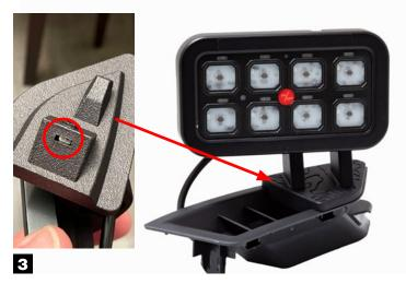
Insert the M3 square nut into the slot, then place your AB8/AB6 mount on the vent nozzle as shown above, sliding the defroster vent fin (in yellow above) into the slot of the mount.
