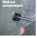
For installing the hardware, the countersunk washer is inserted on the screw, before inserting into the dead pedal. The washers and rubber well nuts are installed as shown above. When installed, the well nut secures the pedal when it is compressed from the screw being tightened, as shown above.
