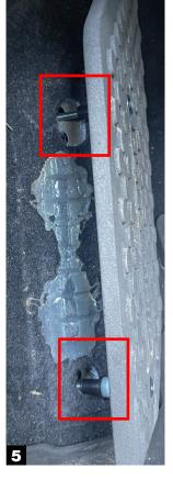
Congratulations! You're on the final step, simply align the screws as shown and insert them into the top and bottom holes, making sure the well nuts also full seat themselves and use the supplied 2.5mm hex key to tighten them down.
