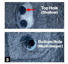
For the holes that the pedal mounts into, it is worth noting the top one is shallow and the bottom one, because of how the carpet is installed, is rather deep. This is why you have the white washers.
