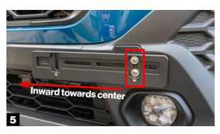
Using the two larger hex head bolts and washers, connect the license plate bracket to the bumper mount. Make sure bracket is mounted inward towards the center of the bumper.
