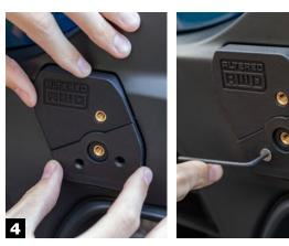
Next, place the locking plate (the smaller 3D printed piece) in place and use the smaller screws and the supplied hex wrench to secure it to the larger printed part. This locks it to your bumper.
