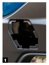
Remove the towing connector cover from the driver side on the front bumper.
