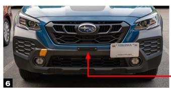
Finally, attach your license plate with the screws that are supplied with the license plate bracket.
