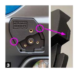
Apply some pressure to the top of the mount and it will seat into place in the bumper opening. There are small snap "tabs" on the sides that help it seat itself.
