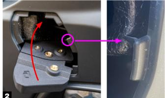
Insert the first part of the license plate mount at this particular angle and then rotate it up vertically as shown above (red arrow).
