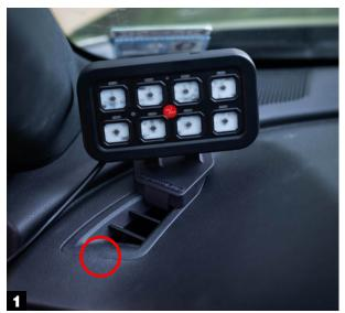
Carefully use an interior panel removal kit, a small flathead screwdriver, or a knife to insert in this area of the vent nozzle and dashboard. Gently pry up the vent nozzle and it will release from the dashboard.
