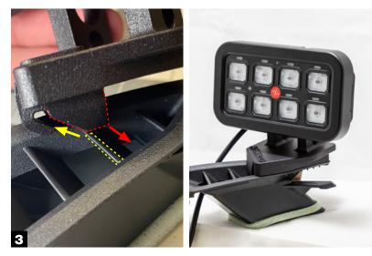
Place your AB8/AB6 mount on the vent nozzle as shown above, sliding the defroster vent fin (in yellow above) into the slot of the mount.
