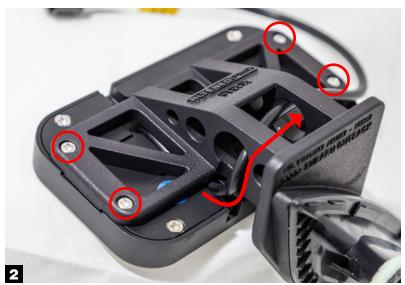
Using 4 screws that came with your AuxBeam controller, install it on the AB8/AB6 mount. Please note the cable routing for the controller, that goes through the mount.
