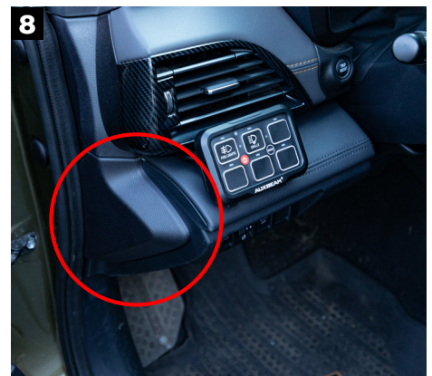
8 Finish the install by closing up the trim panel on the left side and reinserting the fuse panel cover from step 1.
