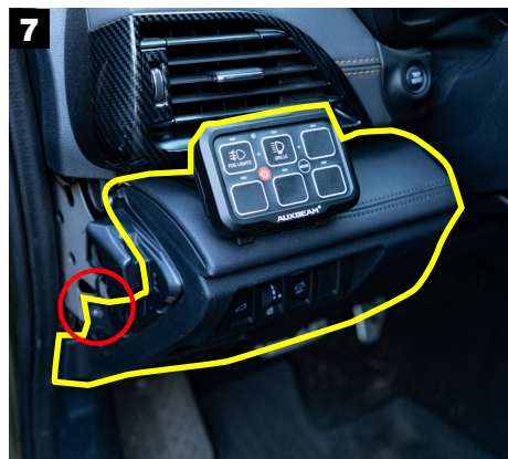
7 Reinsert the dash panel into its clips, firmly pressing it in place. Screw back in the Philips head screw (red circle).
