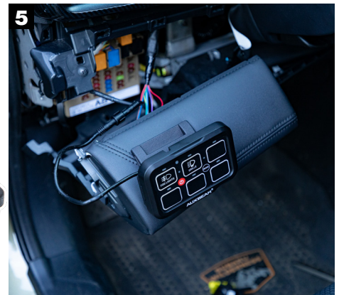
5 Replace the trim panel, clipping it back in and set the MagDash mount onto it. It will magnetically attach, so you can then connect your cable for the AuxBeam panel.
