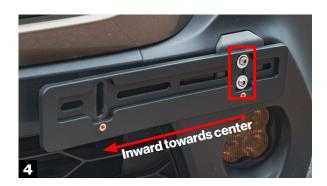
Using the two larger hex head bolts and washers, connect the license plate bracket to the bumper mount. Make sure bracket is mounted inward towards the center of the bumper.
