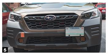
Finally, attach your license plate with the screws that are supplied with the license plate bracket.
