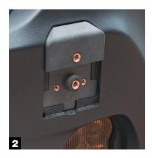
Insert the first part of the license plate mount at an angle and then prop it up vertically as shown above.
