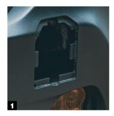
Remove the towing connector cover. You can install this one either the left or right side of your front bumper.
