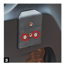
Use the two smaller countersunk hex head screws to secure the smaller part of the plate mount. It will fit snugly. This locks it in place to your bumper.
